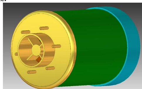
Fig. 2. Three-dimensional model of the reference combustion chamber for numerical investigation
